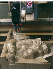
Lion for Ray Kaskey's pediment cut by DSP's Omag CNC five-axis mill.
