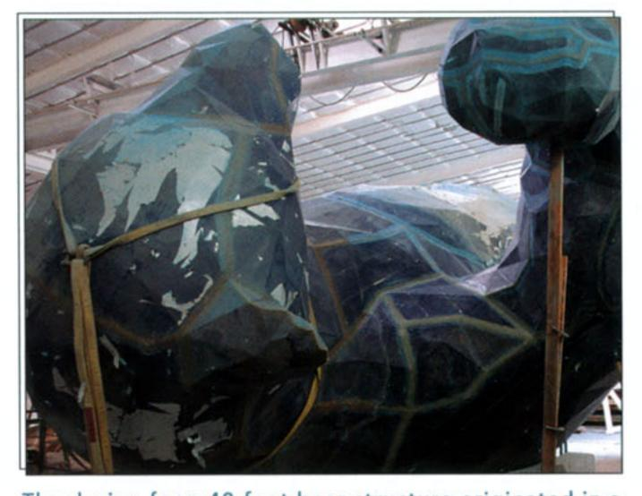
The design for a 40-foot bear structure originated in a 3-D digital model (top) that was later translated into a stereolithographic file to control a CNC miller cutting EPS piecemolds to be covered with foil and gel (middle). The fabricator laid glass fiber and resin over the numerous molds, and assembled them into six final pieces (bottom) for site erection on a foundation.
